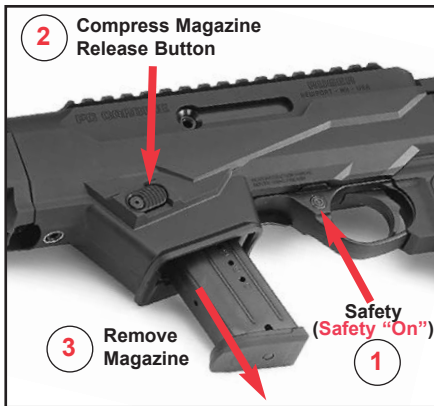
Figure 21. If the hammer is cocked, the safety should be “ON” when the magazine is being removed or inserted. When the magazine release button is pushed in, the magazine is released. Depress the button with your thumb and at the same time grasp the magazine and draw it downward out of the firearm. REMEMBER to check to be sure the chamber is empty after removing the magazine!
